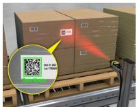
Read 1D and 2D label-based codes on pallets, even codes behind specular wraps.
