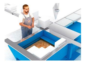
The FAST PICK STATION is a unit consisting of a picking table, chute and film stretcher. It enables goods to be picked onto pallets quickly, in high quality and ergonomically.
