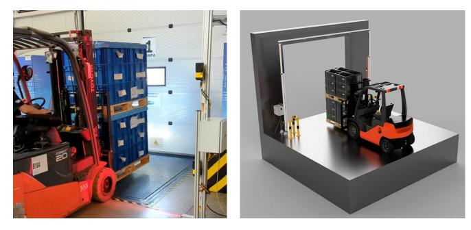
The **AIT SmartGate** is a scangate, for example in the truck loading bay area. It can be used to automatically scan and record all 1D and 2D codes of a pallet on one or two sides.
