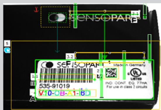
**VISOR® Allround – Object detection in colour plus identification united in one device.**
